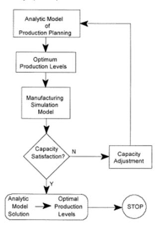
Figure 20: Hybride Simulation Proceedure
