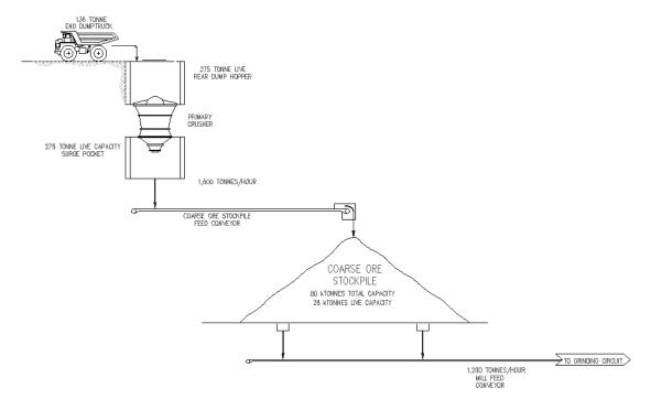
Figure 12: Initial Process Flow sheet
